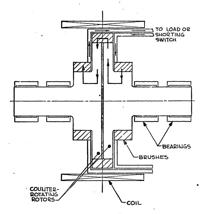
Fig. 3 Fast Discharging Homopolar Machine
